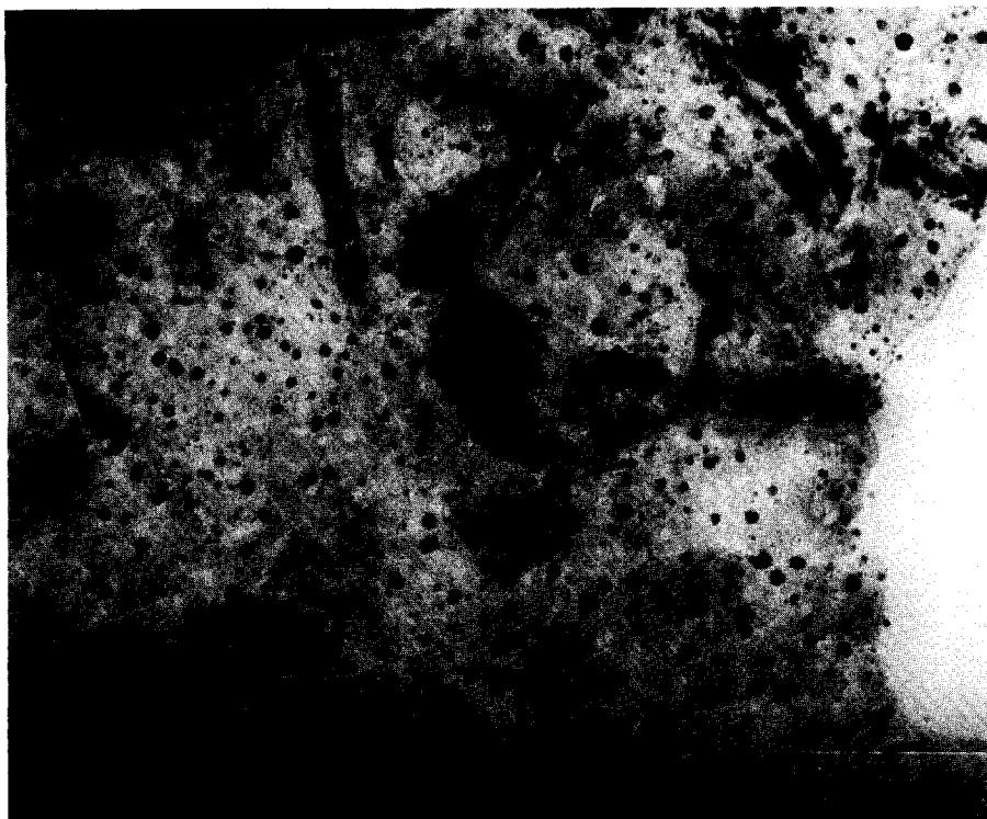
FIG. 6. Transmission electron micrograph showing the effect of burning off of the carbon from a carbon-coated model catalyst. Pt crystallites left tracks and impressions on the alumina surface after the carbon-coated model catalyst was heated for 1 hr at 500°C in O 2 of 10 -2 Torr.
